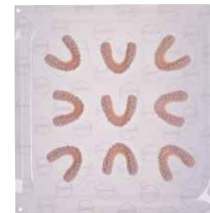
9 blanks in one thermoforming process: Biolon for Vacfomat V9 2.0
