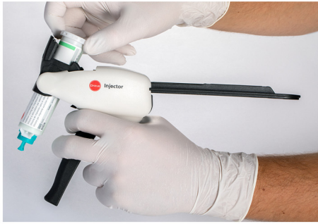
Application of an injector with double cartridge
